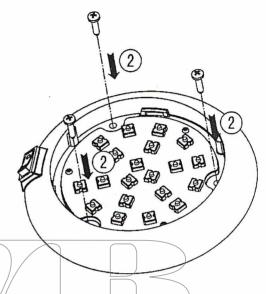
2, Install the Base by fastening 3 screws in place.
