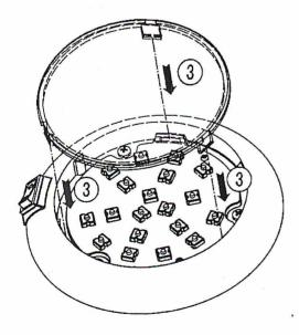
3, Replace the Lens by holding 3 Snap Hooks orientated towards 3 Locking Catches,
