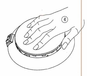
4, Hold the Lens firmly against the Base so 3 Snap Hooks align with 3 Locking Catches; push down the Lens until 3 Snap Hooks are firmly snapped into 3 Locking Catches respectively.
