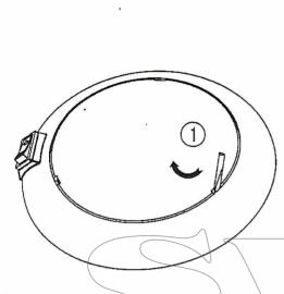
1, Use a slotted screwdriver, gently insert its head into any of 3 Slots on the Lens and pry it to take off the Lens.
