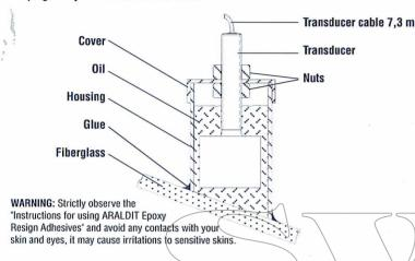
No echosounder will work satisfactorily in an air/water mixture; therefore the greatest care should be exercised to locate the very best mounting position and sometimes several tests may become necessary to obtain the optimum result.
