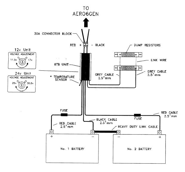
6TB VOLTAGE REGULATOR WIRING DIAGRAM SHOWING CONNECTIONS FOR A SINGLE BATTERY INSTALLATION.
