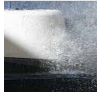
The Broadband family of Radomes have undergone demanding waterproof testing
