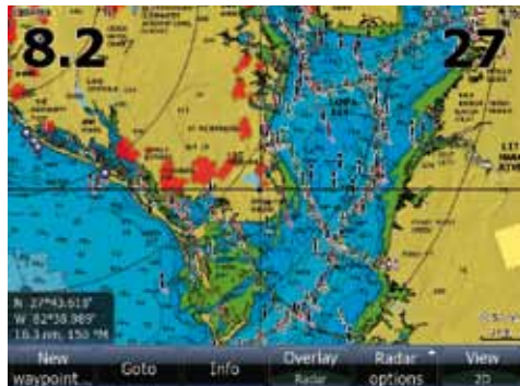
Broadband 4G Radar detects many separated cells inside a Florida rain storm overlaid on a chart greater than 16nm away
