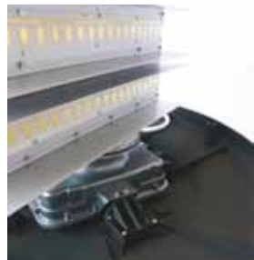
The dual microwave stripline arrays inside of the antenna dome allow continuous transmission and reception, unlike conventional radar that only has one antenna used for both.
