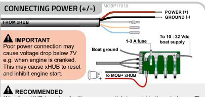
Wire the xHUB to a circuit with a power switch to avoid battery drainage. The xHUB has a power draw of 30mA in idle mode while connected to a power source.
