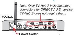
At the rear panel of the TV-Hub, set the power switch to the On position. The TV-Hub supplies power to the antenna. Wait a few minutes for system startup.
