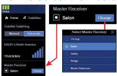
If your system is set up for automatic satellite switching with multiple receivers, you can select the master receiver on the Home page of the web interface. The master receiver controls satellite selection.
