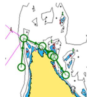
Result after automatic routing
