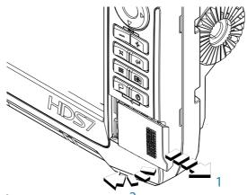
The card reader door should always be shut immediately after inserting or removing a card, in order to prevent possible water ingress
