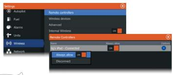
Selecting Always allow will mean the device can automatically connect without needing a password each time. This menu also allows disconnection of devices that no longer require access.
