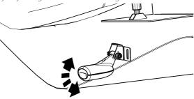
→ **Note:** A transducer that is tilted too far in either direction will not <u>perform</u> well; missing targets, and/or losing the bottom at speed.
