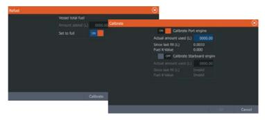
While default calibration is usually accurate enough, it is possible to apply further calibration to accurately match measured flow with actual fuel flow. Access calibration from the 'Refuel' dialog. Calibration is only possible on Navico's Fuel Flow sensor.
