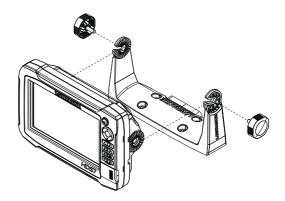
Mount the display to the bracket using the knobs. Hand tighten only. The ratchet teeth in the bracket and display case ensure a positive grip and prevent the unit changing from the desired angle.
