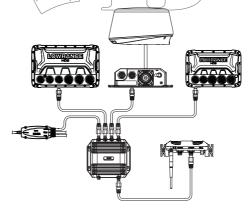
If the number of ethernet devices exceeds the number of available ports on the NEP-2, it is possible to link two or more NEP-2 modules together to provide the required ports. The NEP-2 modules are fitted with 5 ethernet ports.
