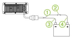
2 If necessary, route a wire ④ between the switch and the battery .
