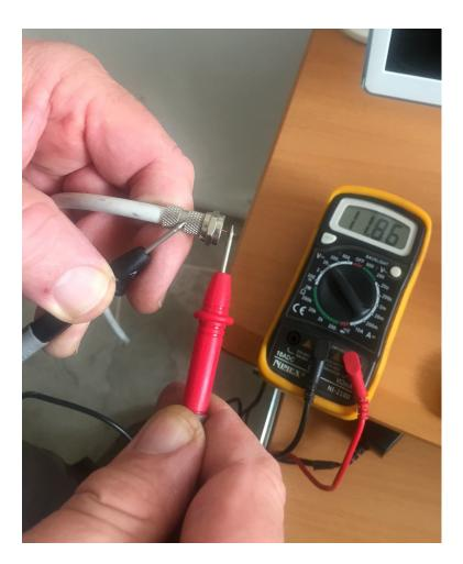
3 - If the antenna regularly gets the 12V then try both outputs by connecting the TV to Output 1 and then to Output 2.
