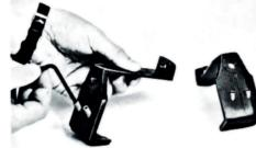
1. Screw the set screws (C) into the brackets, but do not screw them through the plate. Make sure that the screws engage properly in the slanted threaded holes. The latter should be lubricated with grease.
