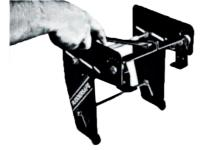
6. Screw the track-bolt (E) about 3-4 turns into the half-brackets. The rudder is now ready for insertion on to the cavitation plate.
