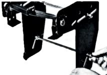
5. Bolt (D) with plastic sleeve is fitted to the rudder blade through hole No.2 (see fig. 2). Fix the other bolt (D) at the topo of hole No.3. When using an engine with a steep propeller pitch, it may be necessary to place the top bolt in hole No.1.
