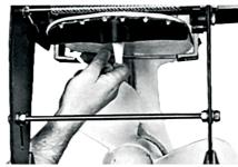
7. Bring the rudder in towards the cavitation plate until the top bolt (D) is up against the cavitation plate. Engage the top cross-stay (B) in the grooves in the bracket.
