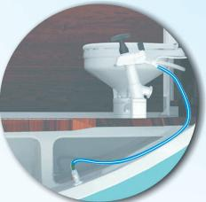
Here's the really clever bit - the really bad smells come from foul water in the <u>inlet</u> hose, so the very thin catheter like sanitizer tube is simply threaded down inside the inlet sanitation hose to the seacock during installation.
