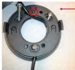
Step 3: Install screws 3 pcs Pull carefully extra cable out .
