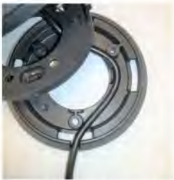
Step 1: Install cable into Wall assembly plate.
