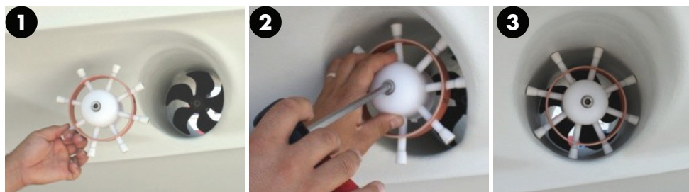
Figure 2 Installation on the side of the tunnel wall
