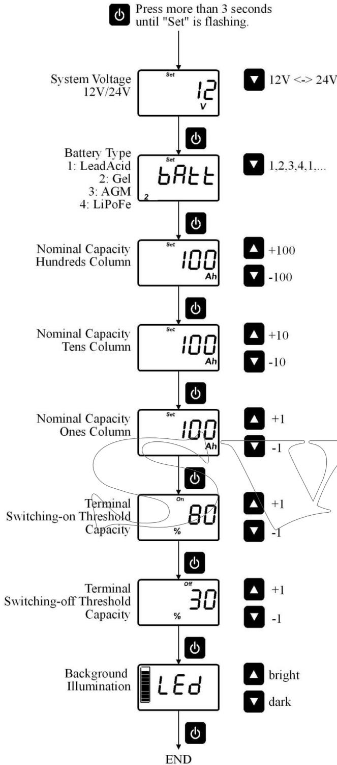
The menu for settings is called by pressing and holding button 3 for more than 3 seconds. The buttons 1 and 2 are used to set the values. In the menu, the button 3 is used to save the setting and to jump to the next menu item.
