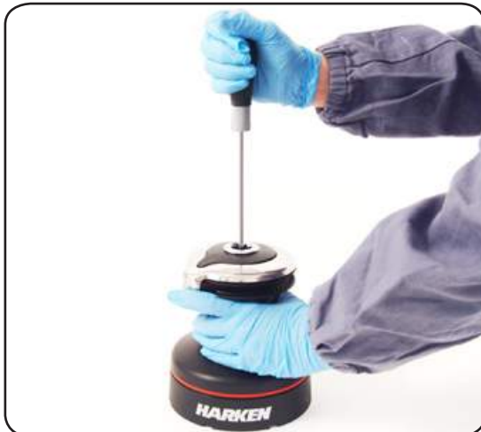
1. Unscrew the central screw ( \approx 2\text{Nm}/18\text{ in-lb} )
