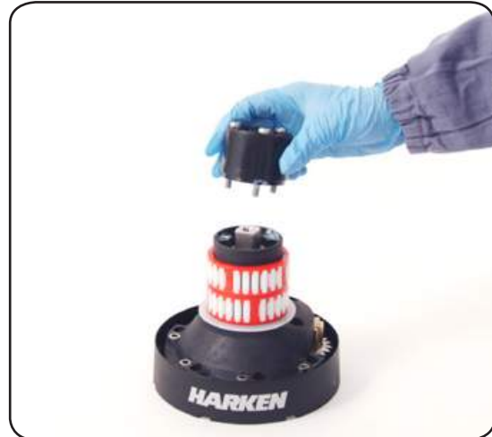
7. Remove the self-tailing arm support n°21 and slide out the bushing
