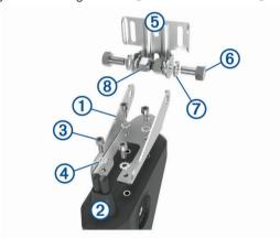
2 Attach the transducer mount bracket to the transom mount bracket (5) using the bolts (6), flat washers (7), and lock nuts
