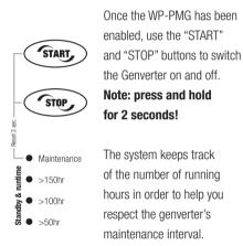
The running hours are shown in increments of 50h. In order to reset the runtime indication (especially after maintenance), press and hold the "START" and "STOP" buttons simultaneously until all four LEDs are extinguished.
